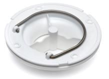
Plastic NOOD water trap for the 59mm S-Series floor gully. The NOOD no-odour water trap is a mechanical odour stop designed to close when there is no water flow, thus preventing odours from escaping through the drain, even when dried out. It is therefore suitable for environments which have little or no water supply for longer periods of time. When water is flowing through, the water trap opens automatically. It can be removed from the outlet gully for easy cleaning and maintenance.
