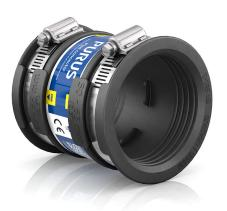
Standard couplings are used to connect two waste water pipes with the same dimension, as well as waste water pipes with the same or different materials and surface structure. Standard couplings are suitable for vertical and horizontal installation. They have two sides, both with hose clamps for external installation of waste water pipes. They are easy to install in a few minutes and are approved for concealed placement. The material is UV-resistant.
