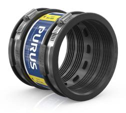
Standard couplings are used to connect two waste water pipes with the same dimension, as well as waste water pipes with the same or different materials and surface structure. Standard couplings are suitable for vertical and horizontal installation. They have two sides, both with hose clamps for external installation of waste water pipes. They are easy to install in a few minutes and are approved for concealed placement. The material is UV-resistant.
