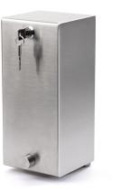
Soap dispenser in 2mm stainless steel for wall installation. Adapted for Tork liquid soap and Tork alcohol / liquid hand soap in 1 litre packaging. The soap dispenser cannot be dismantled without tools and closes tightly to the wall. The design and thickness of the material ensure that the soap dispenser can withstand being damaged without the use of tools, such as kicks, blows and jerks. The soap dispenser has a 10-year anti-vandalism guarantee.
