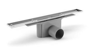
clamping ring, stainless steel frame and installation kit. It is compatible with the 800 Patterned and Limited Edition grates, which are sold separately. The NOOD water trap is a mechanical trap which closes when there is no water present, thus preventing any foul air from escaping through the drain. This linear floor drain can be installed against the wall or elsewhere in the room.
