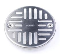
Floor gully Art Deco 130 is a grate made of durable stainless steel. Fits all Purus floor gullies with grate dimension 130mm. The grate is manufactured to ensure a good flow rate and has load class K3. Included with a locking device with a stainless steel locking bracket designed to lock the grate down by attaching to the clamping ring underneath.
