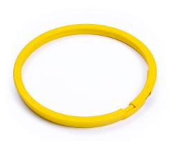
The Clamping ring automatic 150 is made of yellow plastic, fitted with a spring and is used for both sealing membrane and vinyl flooring. It is a self-adjusting clamping ring for vinyl flooring with a thickness of 1,5 mm to 2 mm. Fits in Purus floor drains with a grate dimension of 150mm.
