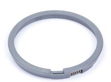
The Clamping ring automatic 130 is made of plastic, fitted with a spring and is used for both sealing membrane and vinyl flooring. It is a self-adjusting clamping ring for vinyl flooring with a thickness of 1,5 mm to 2 mm. Fits in Purus floor drains with grate dimension 150 mm.
