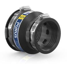
Adaptor couplings are used to connect two waste water pipes with different dimensions, as well as waste water pipes with the same or different materials and surface structure. Adaptor couplings are suitable for vertical and horizontal installation. They have two sides, both with hose clamps for external installation of waste water pipes. They are easy to install in a few minutes and are approved for concealed placement. The material is UV-resistant.
